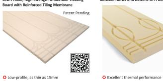
Ideal for refurbishment applications Fits between timber joists or battens O Directly accepts floor tile Manufactured to suit pipe and spacing required Ultra high compressive strength - 500kPa O Robust Detail FFT2 compliant component High thermal performance 30, 40, 50mm x 300mm x 1250mm Manufactured to suit pipe and spacing required **15, 18, 20, 25mm** x 600mm x 1200mm
