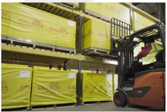
**ScreedBoard®** is supplied on pallets, wrapped in temporary protection. This covering is to offer dust protection and a temporary measure to protect the boards from the weather during the loading/unloading process, it is **not** a waterproof cover.
