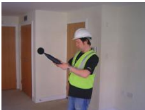
Airborne sound tested to BS EN ISO 140-4 1998
