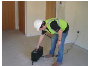
Impact sound tested to BS EN ISO 140-7 1998
