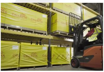
HiDECK® Structural, XFLO® JB and timber battens are supplied on pallets, wrapped in temporary protection. This covering is to offer dust protection and a temporary measure to protect the boards from the weather during the loading/unloading process, it is not a waterproof cover.
