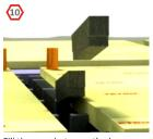
Fill the gaps between the beams with concrete closer blocks and slip bricks
