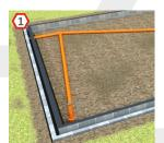
Build up the foundation walls to the desired height & install a suitable damp proof course
