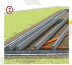
Using the beam layout provided, carefully place the beams across the floor at the specified centres
