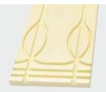
CELLECTA's XFLO JB boards are manufactured from 100% recyclable HEXATHERM, using a CNC to route out the pipe diameter and centres required. The board's are made to suit the specific batten spacing. When used in conjunction with CELLECTA'S ULTRAplates (heat diffuser plates) will provide outstanding heat output.
