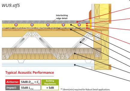
**CELLECTA ScreedBoard 20** Highly conductive interlocking floorboard
