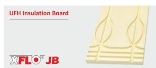
CELLECTA's XFLO JB boards are manufactured from 100% recyclable HEXATHERM, using a CNC to route out the pipe diameter and centres required. The board's are made to suit the specific batten spacing. When used in conjunction with CELLECTA's ULTRAplates (heat diffuser plates) will provide outstanding heat output.
