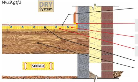
Floor finish (Ceramic / stone floor tiles or engineered timber flooring)
