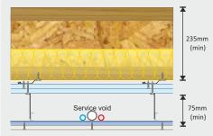
Sound absorbing quilt fitted between joists 50mm CELLECTA FIBREfon Micro 50 100mm (min) mineral wool quilt -10-33kg/m
