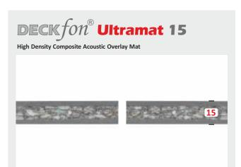
**DECKfon Ultramat 15** high performance, three layer composite mat that will improve both the impact and airborne performance of a floor where there is limited room height available. Once laid, the mat can be covered with carpet or suitable wooden flooring
