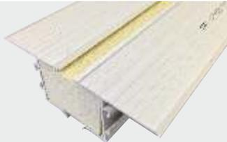
**XCPL** combine the benefits of a **HEXATHERM®** extruded polystyrene with one or two U-PVC damp proof course profiles to produce a rigid cavity closer that eliminates cold bridging around window and door openings.
