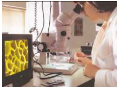
The closed-cell structure of YELOFOAM magnified by 500 times.
